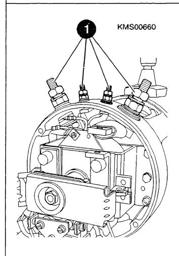
ASSEMBLING STARTING-MOTOR SOLENOID WITH CONTROL RELAY
